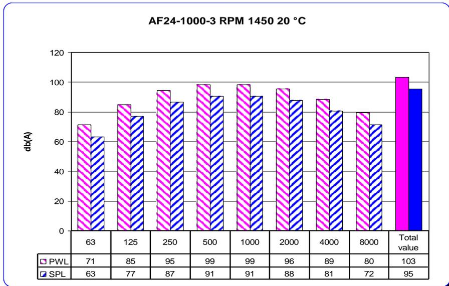
Noise spectrum referring to max efficiency of 20° curve
